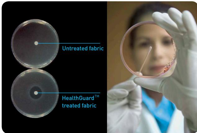
The petri dishes above show the difference between a HealthGuard treated sample and an untreated sample. The surroundings of the HealthGuard treated fabric were resistant to *Staphylococcus aureus* MRSA A129 to a distance of 6mm.
